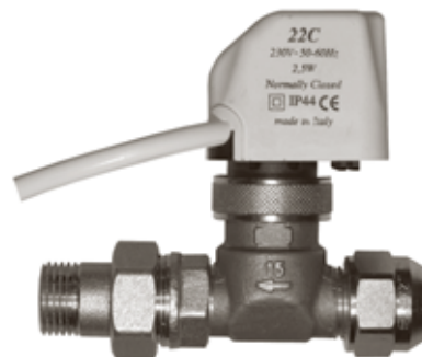
06 The two-position line valve R1/2", R3/4" with two connections is easy to connect to the piping network. The valve is operated by an electric-thermal drive with "ON-OFF" control.
