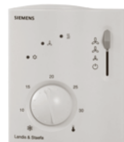
012B Room thermostat - automatic heating/cooling switching - fan speed selection switch (MIN-MED-MAX) - for 4-pipe systems - wall installation
